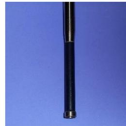
Thermal Instrument is utilizing our base model 62-9 single piece insertion probe at this location. The meter has a protective polymer coating applied to the
